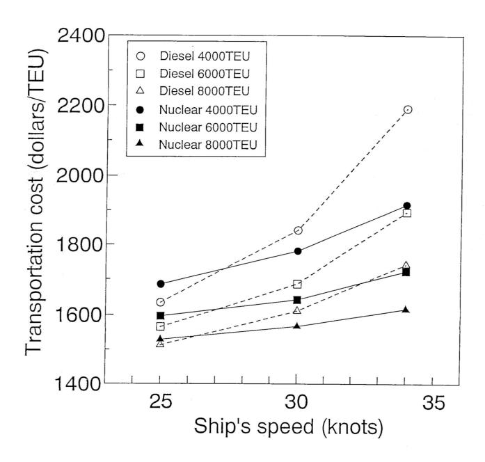
Figure 2.3 Cost evaluation of nuclear ships on the Pacific Ocean
