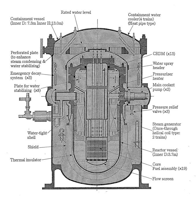
Figure 2.1 Conceptual schema of Marine Reactor X
