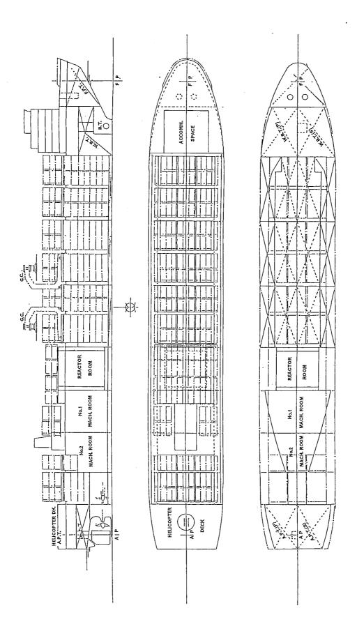
Figure 2.5 General arrangements of the nuclear icebreaking container ship model
