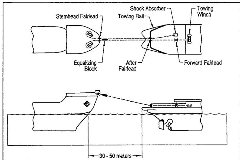
Tandem tow can be performed if the stern of the icebreakers has a stern notch and the towed vessels are sufficiently strengthened in the bow. Every icebreaker on the NSR is equipped with stern notches and the method has been much used since the early eighties. Also the SA-15 merchant vessels are equipped with a stern notch, which makes it possible to tow
