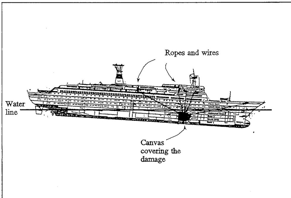
Figure 2.19 The hull damage on the "Maxim Gorkiy" was preliminarily repaired by divers after collision with ice in the Svalbard area 1989 (Source: Norwegian Coast Guard).
