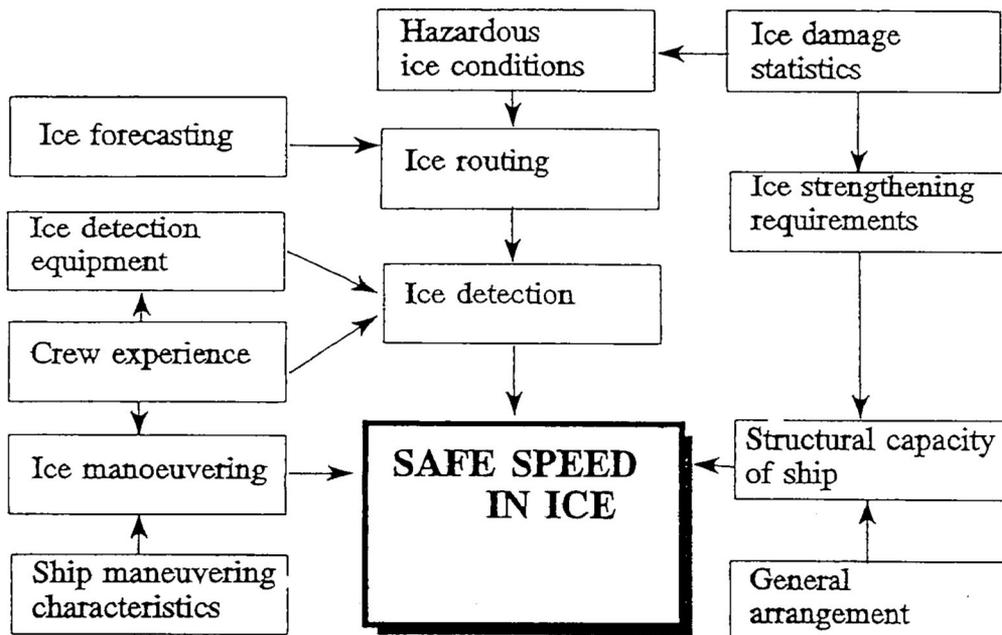
Figure 2.15 Important elements in determining safe speed in ice (Køhler, 86)
