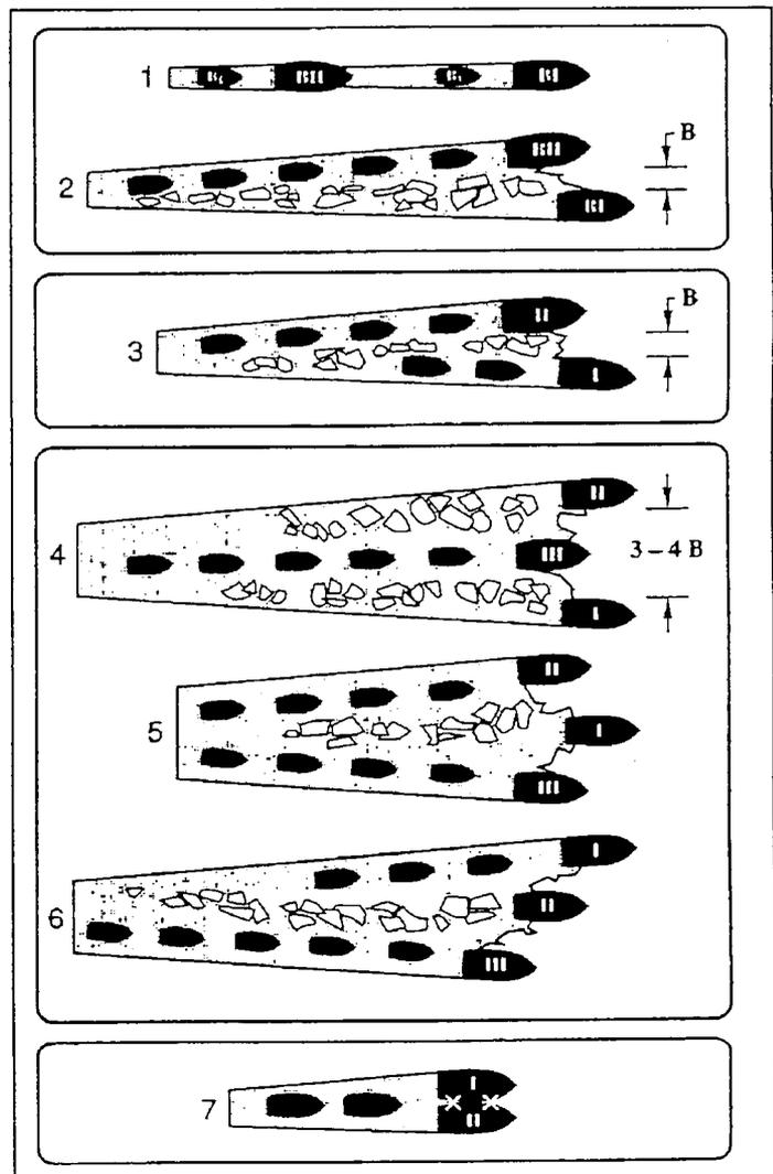
A clean and easy navigable channel depends very much on the shape of the icebreaker. Traditionally, this has been a matter of the beam of the hull. New development on bow shape has proved that the icebreaker performance can be improved significantly. An example of this is the Thyssen Waas bow build on the icebreakers Kapitan Sorokin and Madyug. On figure 2.11 this improvement is clearly illustrated in level ice where the advantages are most significant.
