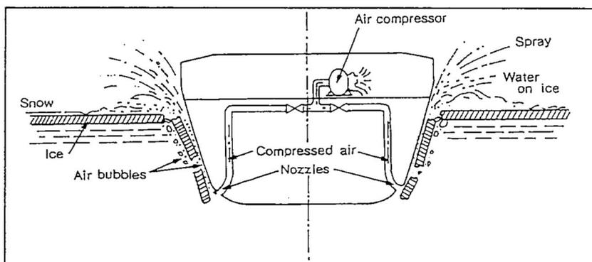
All Rossiya- and Taymyr class icebreakers and the merchant ships of the SA-15 type (Norilsk-class) are equipped with an air bubbling system.
