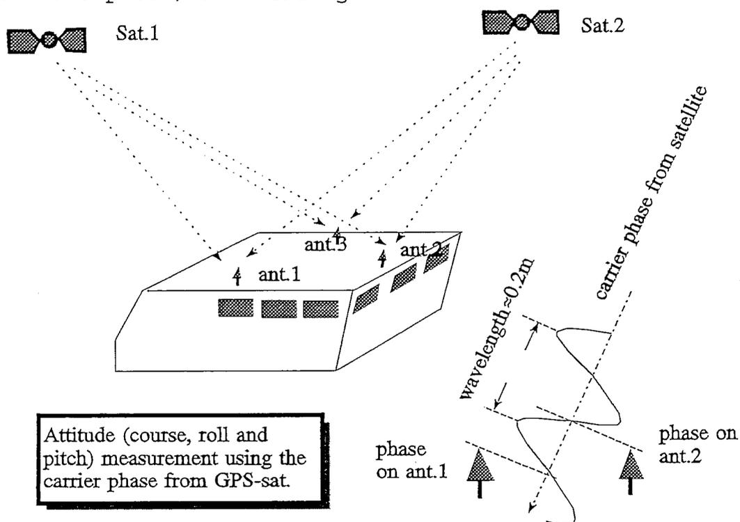
Figure 1.20 By means of 2 or more antennas the GPS can be used for attitude determination (course, roll and pitch), important when navigating in Arctic areas where compasses often are incorrect.
