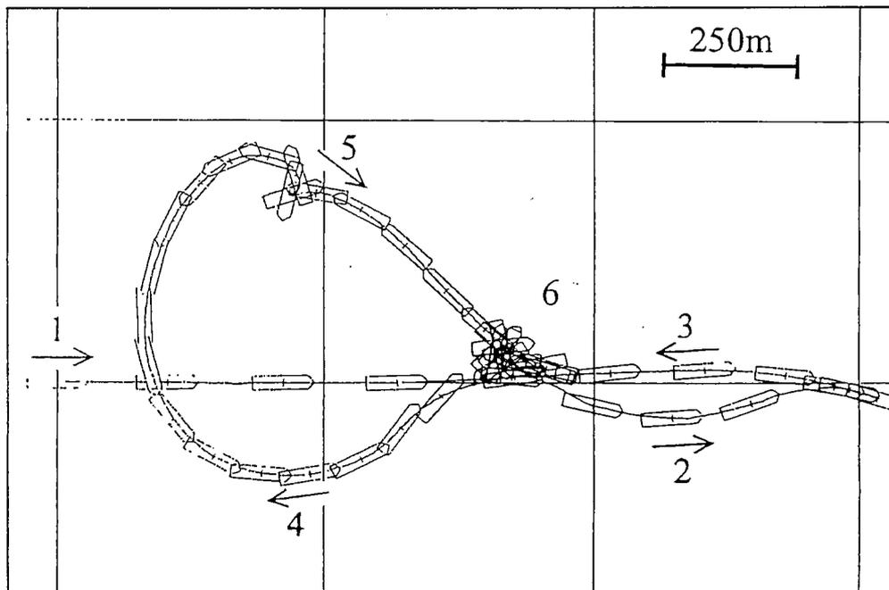
Figure 2.4 Equipped with 2 azimuth thrusters the Finnish icebreaker "Fennica" has eminent maneuverability (Savikurki, 93).
