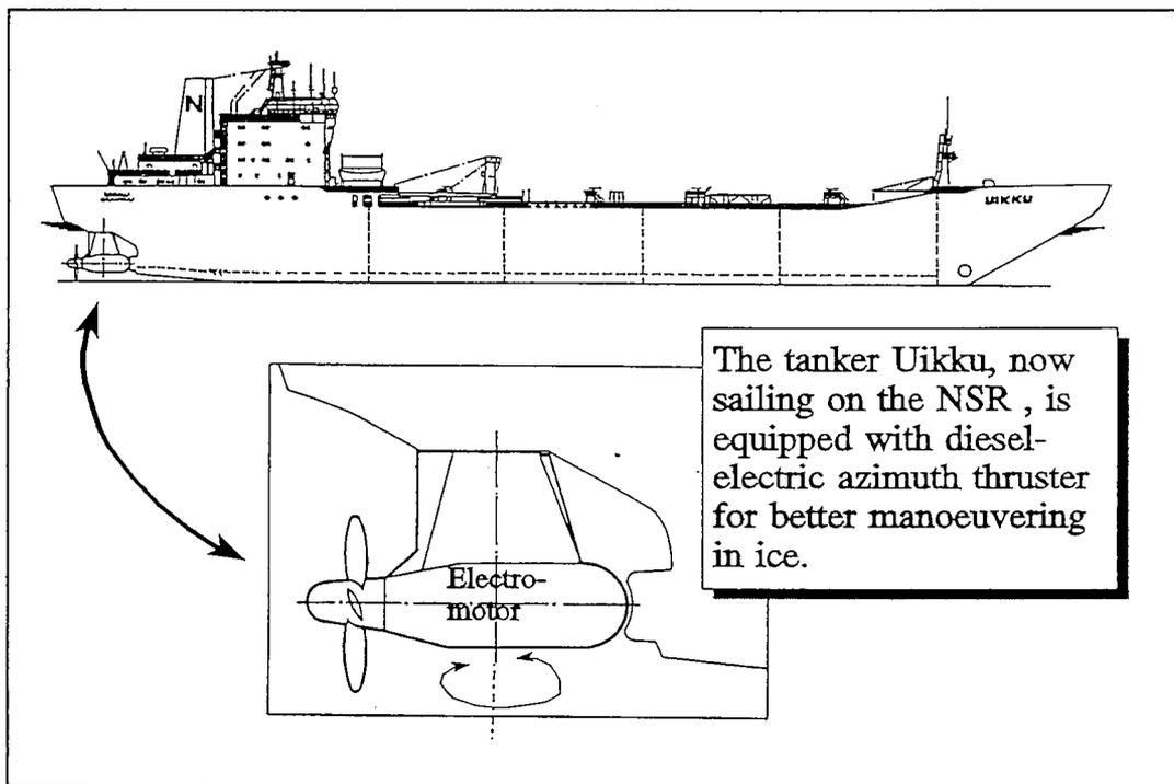
*Figure 3.10* Azimuth thrusters have shown very promising results on the new Finnish icebreakers. Here shown on the tanker Uikku (Source: Kværner Masa Yard).
