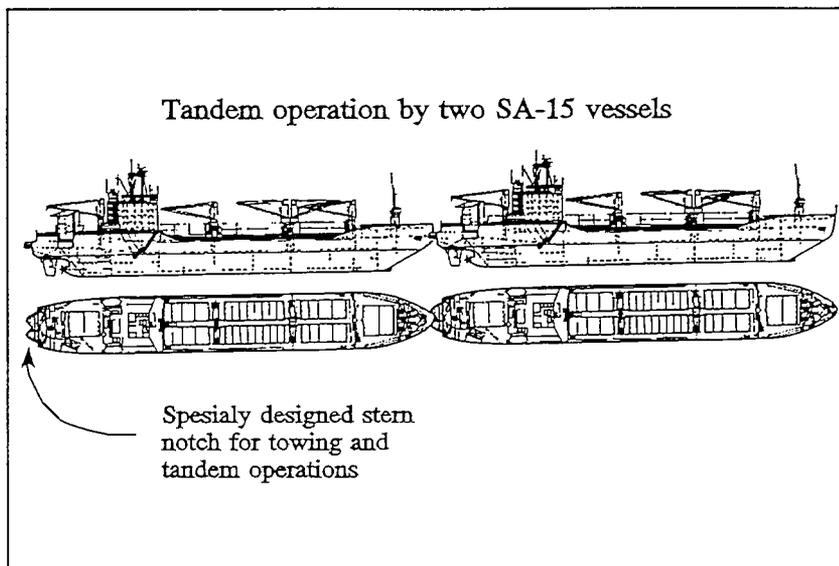
The tandem concept has been studied as a tanker project for taking petroleum resources out of the Arctic. One of these projects is shown in figure 2.14.
