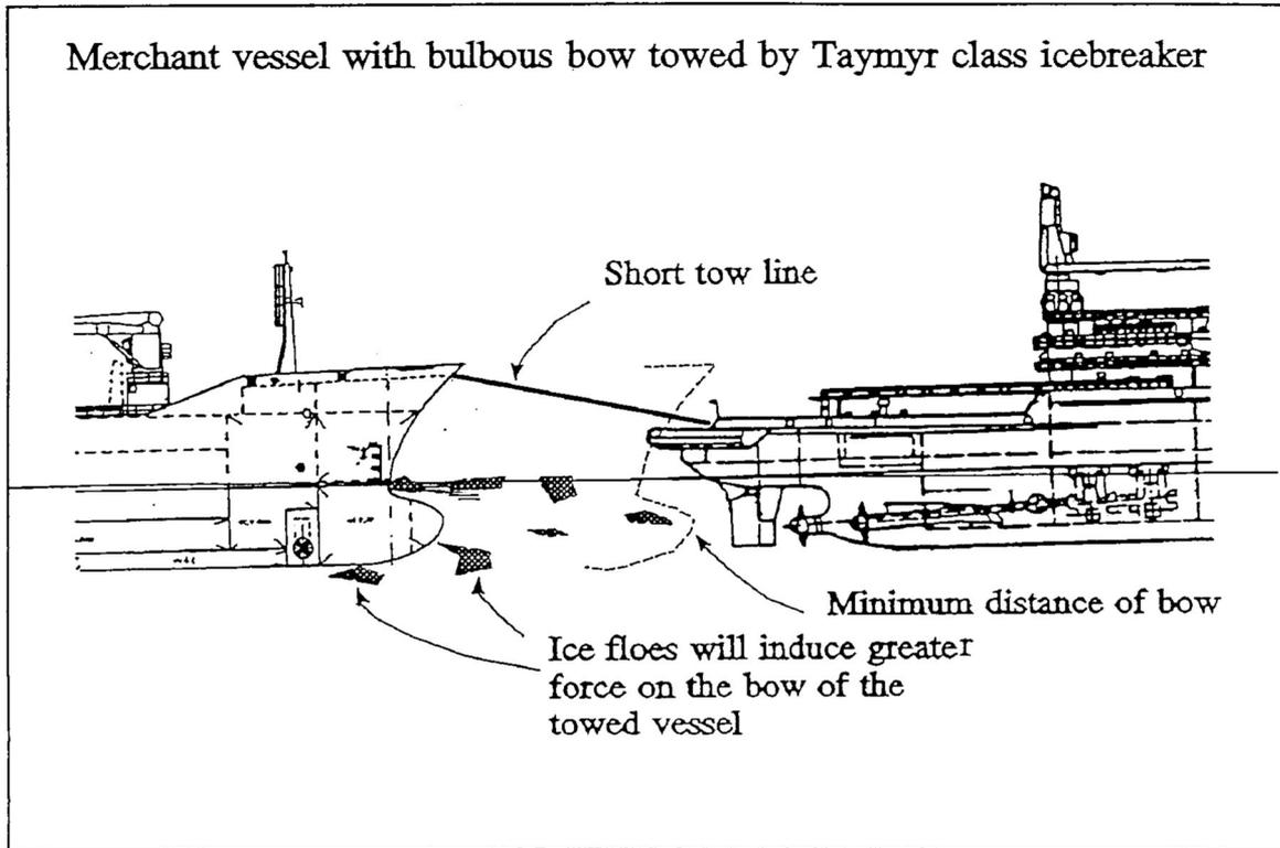
Figure 3.1 Merchant vessels with bulbous bow will normally not be given permission to sail the NSR due to extreme loads during close tow operations after icebreakers.
