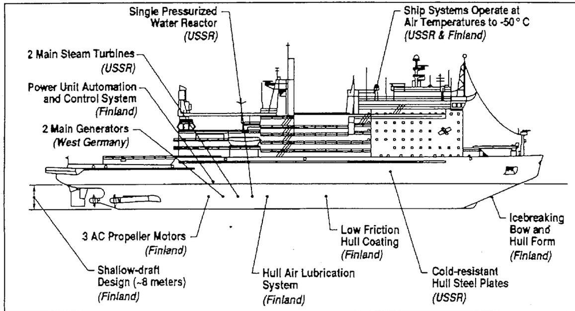
Figure 3.11 Shallow draft nuclear icebreaker of Taymyr class with relevant system for high performance icebreaking (Brigham, 91)
