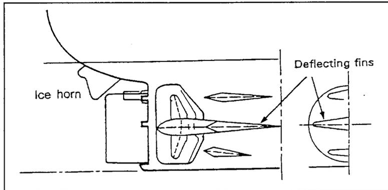
Some icebreakers with two rudders like the Swedish Oden are equipped with rudder stops. None of the Russian Arctic icebreakers are equipped with more than 1 rudder. Ships equipped with azimuth thrusters are not equipped with rudder (fig.3.10)
