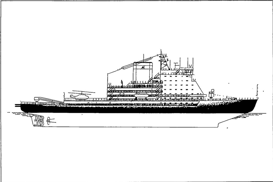
Figure 3.12      *The new diesel-electric icebreaker concept called the Anadyr type is planned to replace the Moskva- and Yarmak-type icebreakers early in the next century.*
