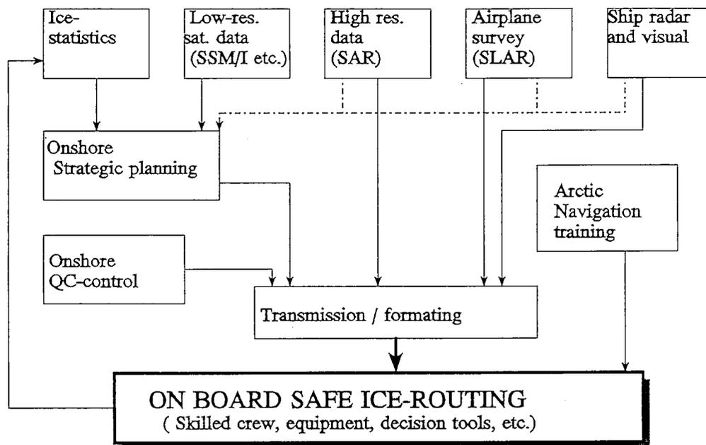
*Figure 1.2* Important elements in the routing process. Note that the need of high resolution and detailed information increases as the execution gets closer.
