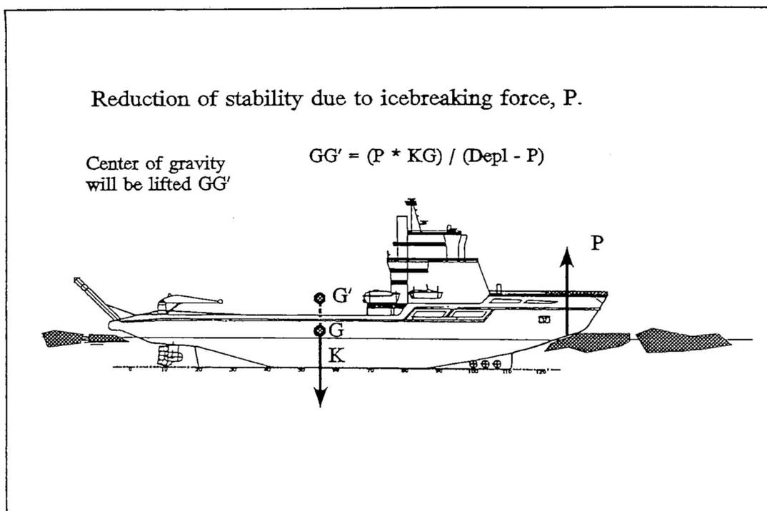
*Figure 2.22 A ship's center of gravity will be raised during icebreaking and the stability will be reduced.*
