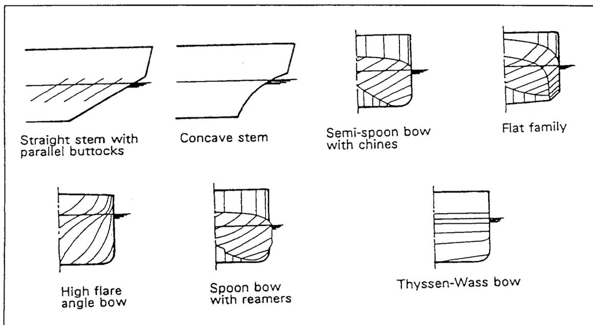
Figure 3.4      *Different bow form features on ice-going vessels (CCG,92).*
