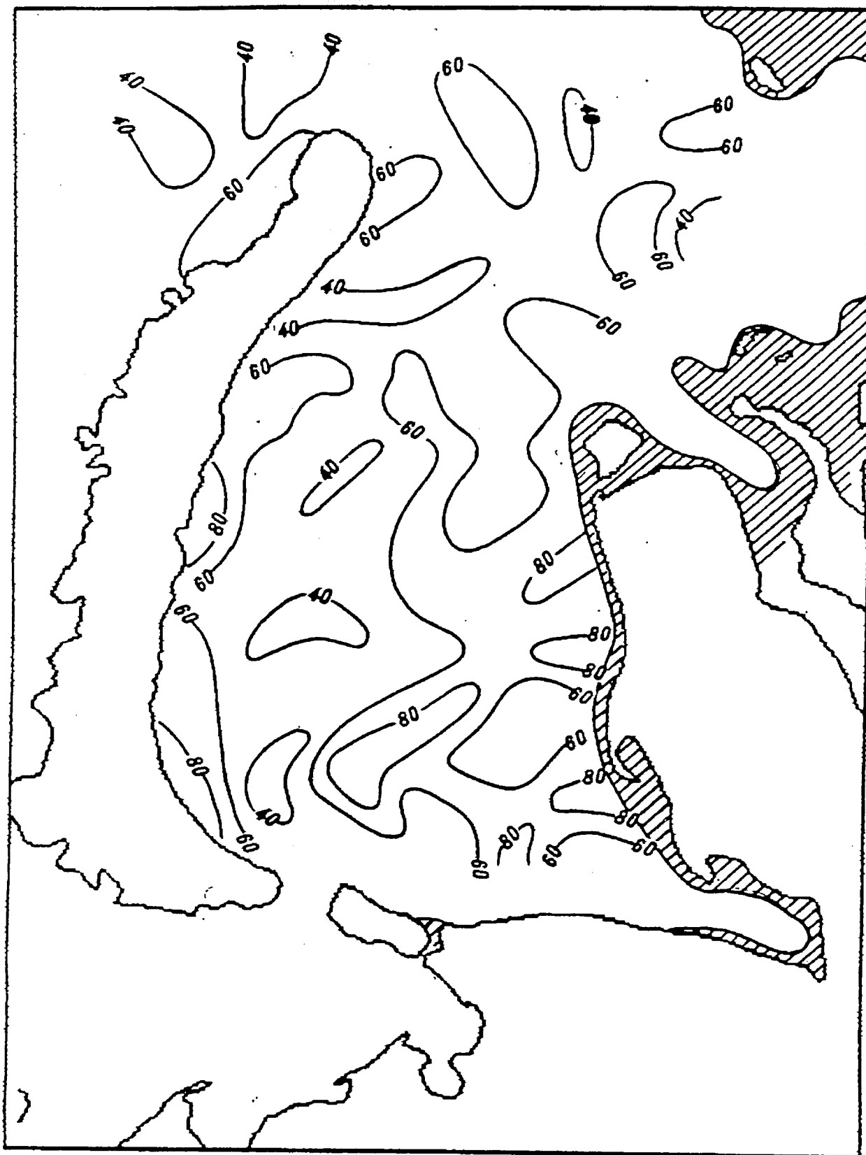
Fig. 7. Occurrence frequency of a modal interval of orientation of discontinuities in ice cover of the south-western Kara Sea in April on the basis of data for 5 years
