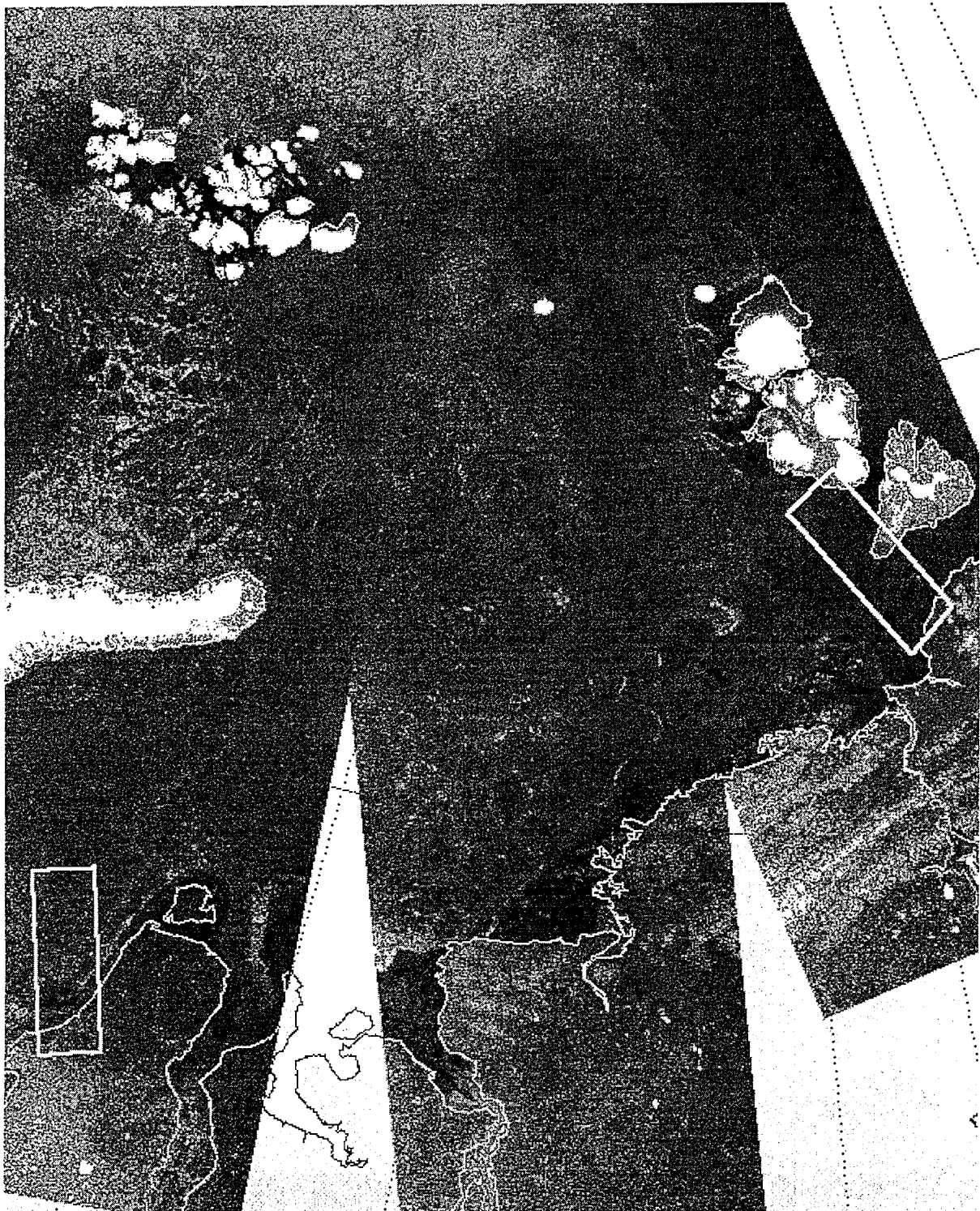
Figure 10. Digital mosaic of SLR images in the Kara Sea presented in a polar stereographic projection, obtained from Okean N7 in May 16 - 21 1996. The white rectangles mark the locations of two ERS SAR images obtained at the same time. Image courtesy: NPO Planeta, Department of thematic Processing.
